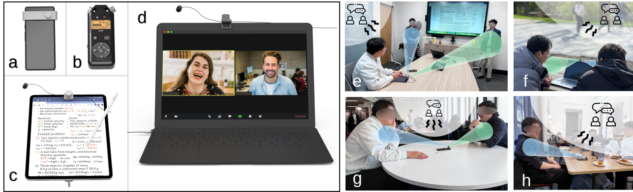
Figure 16: Applications of SonicSieve. (a–d) Our system can be physically connected to various computing devices with a microphone jack including smartphones, handheld digital voice recorders, tablets, and laptops. (e–h) SonicSieve can be used in various application scenarios including (e) Transcribing a presentation with speaker attribution. (f) Conducting a remote meeting by a noisy park. (g) Recording a podcast without specialized soundproof booths. (h) Interacting with an AI voice assistant in a noisy restaurant.
